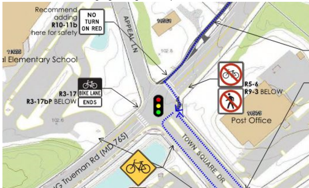
Figure 10 – Intersection of HG Trueman Road (MD 765) at Town Sq Dr – Design Option A (Signage References are to Maryland-MUTCD sign manual – latest edition)
